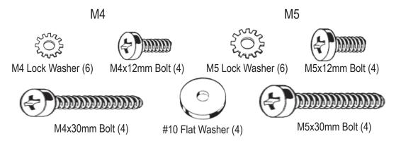
Hardware for securing bracket: Select the appropriate length based on the thickness of your mounting surface.
